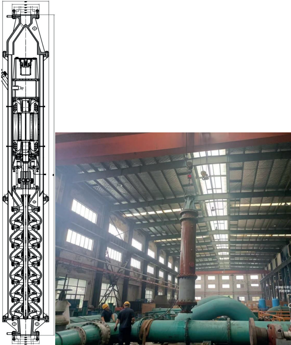
Fig. 4. Overall design of the six-stage pump (2020-2023)
