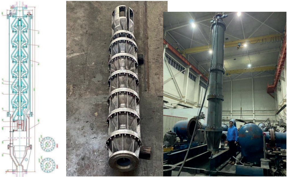
Fig. 3. Overall view and manufacturing of a six-stage pump (2015-2020) (right, author)
