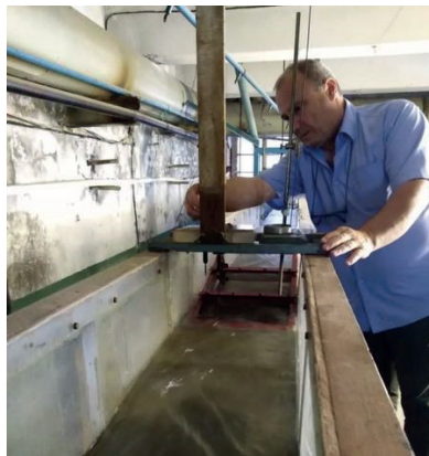
Figure 7 Debris flow regulation elastic barrage during the laboratory tests
