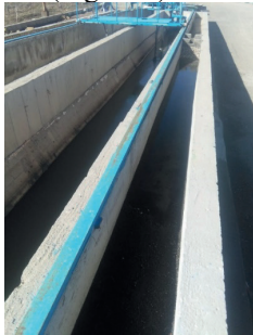
Figure 1 Experimental setup for a rectangular concrete channel (upstream view)
