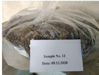
Figure 3 The sediment sample prepared for gradation test (each sample has 2kg weight)
